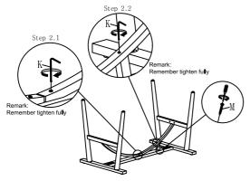
Step 3: Attach Center Rail E with Table Leg B by insert (G,J & K)
